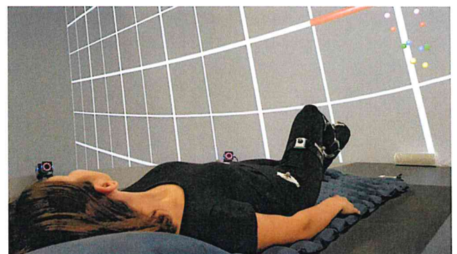
Figure 4: supine exercise with Re.Flex sensors and Vicon Markers placed on the affected joint
